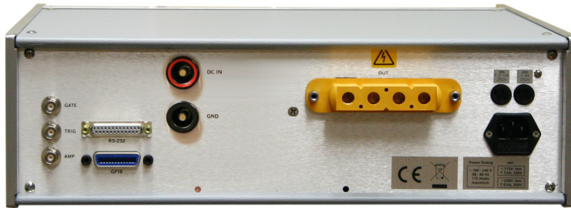
AV-109F Series Rear Panel. (AV-109E models do not have the DC and GND power supply terminals).
