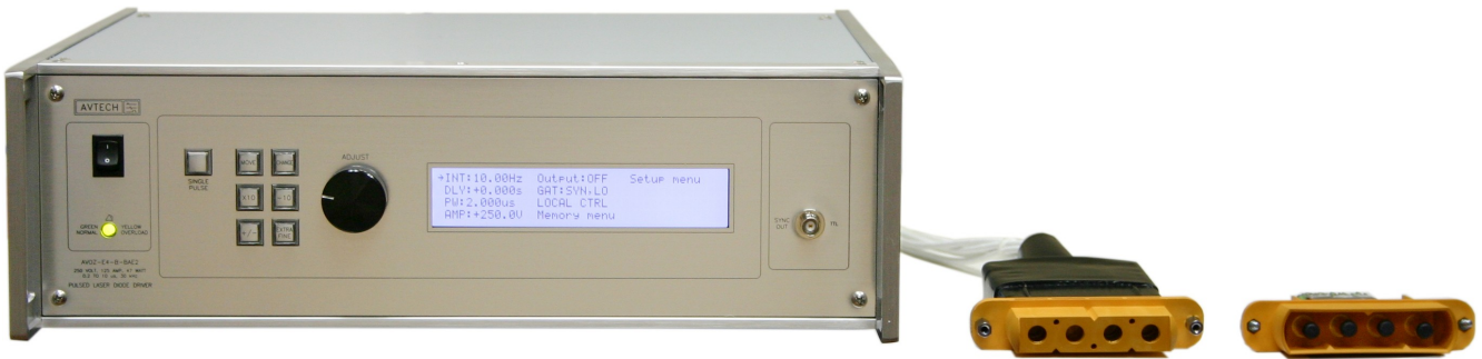
Pulsar mainframe (left) with AK9 kit, including the AV-HLZ1-100 output cable (middle) and mating adapter (right)
